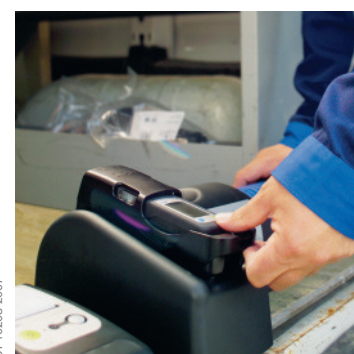
Dräger X-am® 2000 Optional Dräger Bump Test Station for an efficient Bump Test under 10 seconds.
