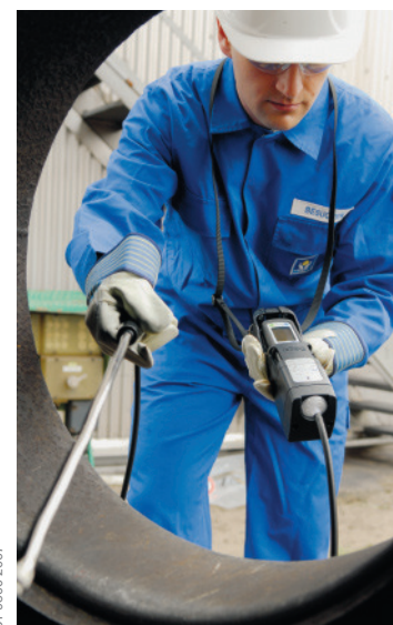
Dräger X-am® 2000 Flexible with an external pump for confined space entry.
